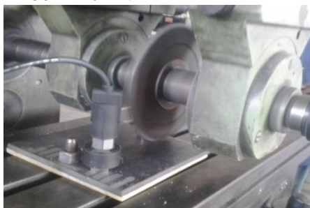
Figure1. mild steel plate placed on composite plate bolted to slotted table of milling machine
